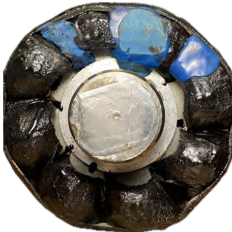
Figure 4.8: Image of the prototyped rotor post-application of epoxy resin, fiberglass bandage, and extra material for balancing.
