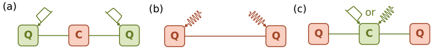
Figure 4.1: Three types of two-qubit coupling scheme. Fixed-frequency and tunable elements are represented by green and red blocks, respectively. (a) Tunable qubits coupled via fixed resonator coupler. (b) Fixed-frequency qubits with gate activated by microwave drives. (c) Fixed-frequency qubits coupled via tunable coupler.
