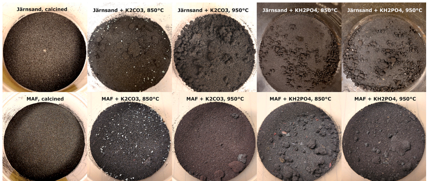
Fig. 4. Photos of the samples, exposed to 21 reduction-oxidation-cycles and K_2CO_3 or KH_2PO_4 .
