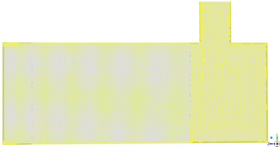
Fig. 8. Cut section along the mid-plane of the computational domain, illustrating the mesh resolution inside and upstream the catalyst region. The flow enters from the vertical duct and exits towards the left.
