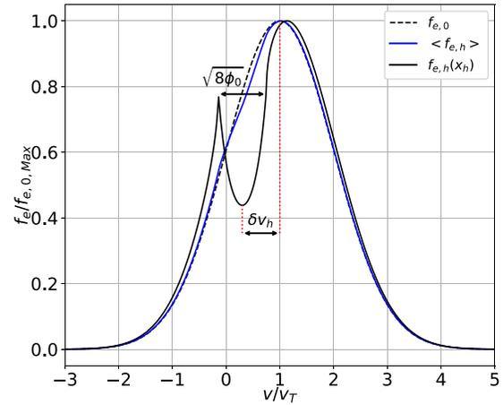
FIG. 1. Electron Schamel distribution function slice at  $x = x_h$  normalized to the maximum of the electron equilibrium distribution function  $f_{e,0,max} = n_{s,0}/v_{e,T}\sqrt{2\pi}$ , for a mass ratio of  $m_i/m_e = 36$ , and parameters  $\phi_0 = 0.10$ ,  $\beta_h = -5.80$ , and  $\delta v_h = 0.70v_T$ .
