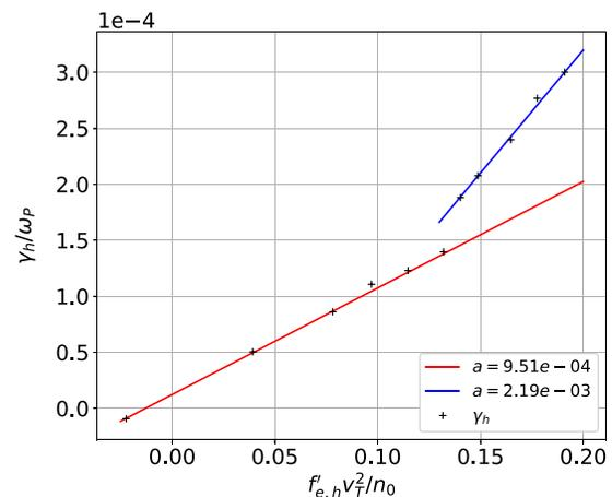
**FIG. 7.** Electron-hole phasetrophy growth-rate as a function of the electron equilibrium distribution gradient at the average hole velocity at the moment of the measurement. Growth-rate from numerical simulations in black crosses and linear fittings of the data in solid red and blue lines.
