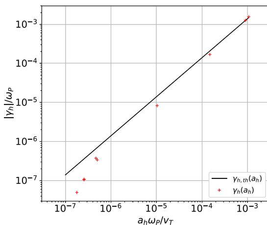
**FIG. 6.** Log-log plot of the absolute value of the growth-rate of the electron-hole's phasetrophy as a function of the electron-hole's acceleration. Black line: Analytical expression (14). Red crosses: measurements from numerical simulations.
