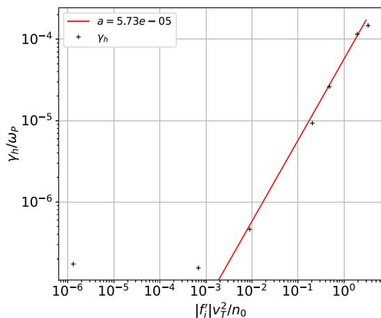
**FIG. 8.** Electron-hole phasetrophy growth-rate as a function of the absolute value of the ion equilibrium distribution gradient at the average hole velocity at the moment of the measurement. Growth-rate from numerical simulations in black crosses and linear data fitting in the high amplitude regime in the solid red line.
