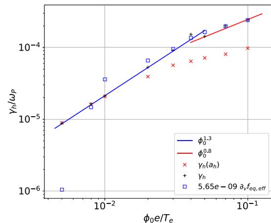
**FIG. 9.** Electron-hole phasetrophy growth-rate as a function of the initial amplitude of the electric potential. Growth-rate from numerical simulations in black crosses,  $\gamma_h(a_h)$  is the growth-rate calculated from the acceleration, linear data fitting in the low and high amplitude regime in solid red and blue lines, and the effective electron equilibrium gradient normalized to the data in blue squares.
