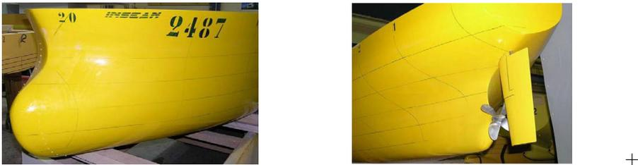
Figure 4.9: Ship model used in HSVA and MARIN model tests. Copyright HSVA.
