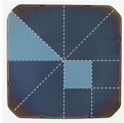
Fig. A2: Division of the flexible CIGS solar cell ( $15.6 \times 15.6 \text{ cm}^2$ ) into smaller pieces which were used in the experiments: triangular ( $30.4 \text{ cm}^2$ ) and square ( $15.2 \text{ cm}^2$ ) pieces for the acid and alkaline leaching experiments, respectively.
