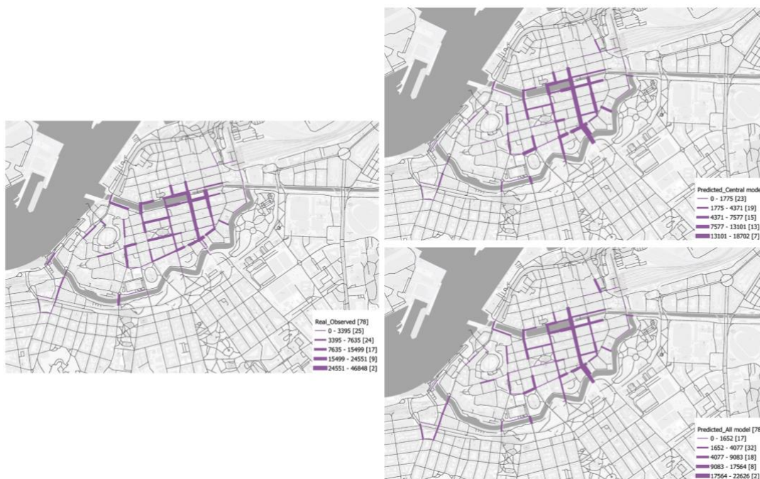
Figure 4: Relative distribution of observed counts (left) vs relative distribution of predicted counts for the STHLM Central (right, top) and STHLM All (right, bottom). The legend ranges show number of pedestrians. In brackets is the number of street segments per range.
