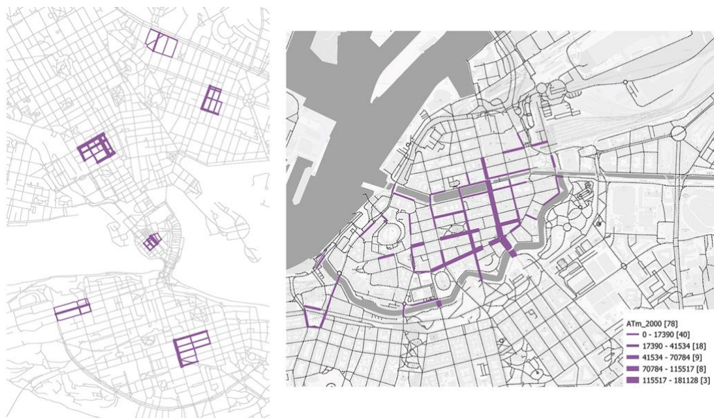
Figure 9: Attraction Betweenness centrality weighted for Local markets in the 6 central areas in Stockholm training data (left) and in the observed streets in Gothenburg (right)
