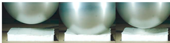
Fig. 5. Drop test (-6 ms, 4 ms and 40 ms). Observe the permanent deformation in unloading.
