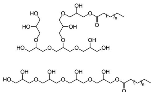
Fig. 5 Fatty acid ester of oligomeric glycerol. For the surfactant used in the food industry the value of  $n$  is typically around 3 but the oligoglycerol chain has a broad homologue distribution. The polyglycerol moiety can exhibit different degrees of branching.
