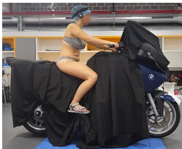
Figure 2. Volunteer seated on the touring motorcycle (MC), with the vehicle covered to prevent measurement interference.
