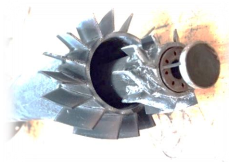
Figure 9. Photograph of the combi-burner used in the Chalmers Unit. The centre hole is for lignite injection, the surrounding holes are for propane, and both outer registers with blades is for the primary air with swirl.
