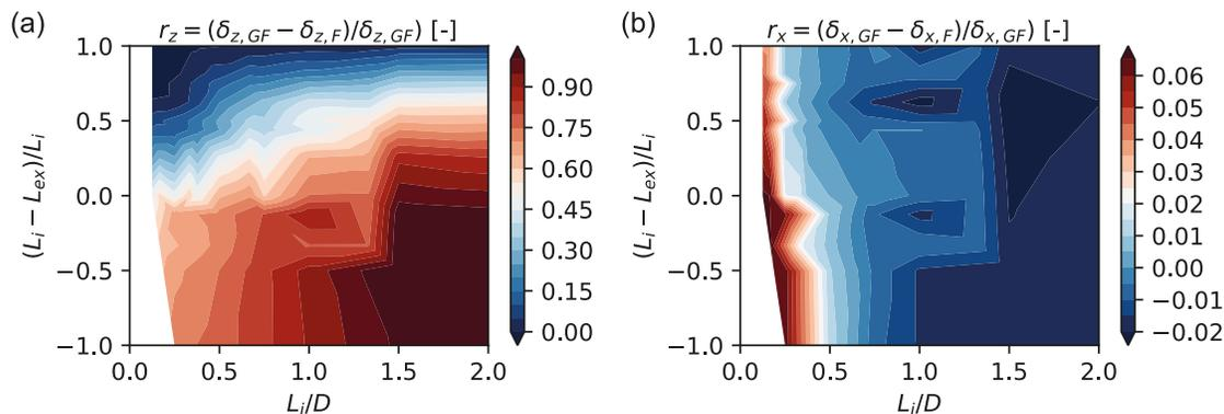
**Fig. 12.** Influence of geometry on the tilt and deflection ratio of the slab of an existing foundation (F) relative to the greenfield (GF) situation: (a)  $Tilt_F/Tilt_{GF}$  (-),  $L_i = 40$  m; (b)  $DR_F/DR_{GF}$  (-),  $L_i = 40$  m; (c)  $Tilt_F/Tilt_{GF}$  (-),  $L_i = 60$  m; (d)  $DR_F/DR_{GF}$  (-),  $L_i = 60$  m; (e)  $Tilt_F/Tilt_{GF}$  (-),  $L_i = 80$  m; (f)  $DR_F/DR_{GF}$  (-),  $L_i = 80$  m.
