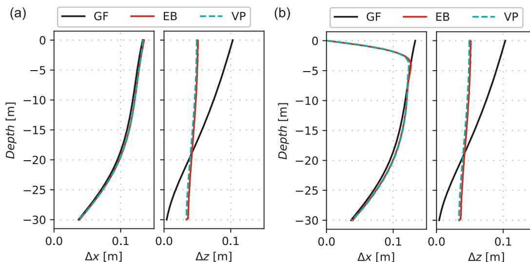
Figure 3 shows that the EB predicts, for the numerical modelling approach considered, similar deflection behaviour as the VP when using a fixed or a free moving pile head as boundary condition. Furthermore, the displacements of the soil surrounding the pile in the case of a laterally fixed pile head are presented in Fig. 4. Also in this case, the soil displacements are largely similar when comparing the response from the VP and the EB.
