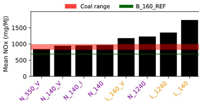
Fig. 6.  $\text{NO}_x$  emissions levels (in mg/MJ) ordered chronologically, with the coal reference range in red and the reference combi-burner in green. In plot (b), orange is used to represent the “L” cases, while purple represents the “N” cases. (For interpretation of the references to colour in this figure legend, the reader is referred to the Web version of this article.)
