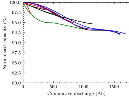
**Figure 3.6:** Normalized capacity fade curves of NMC/graphite-SiO<sub>x</sub> cells in the Stanford Energy Control Lab dataset [79].
