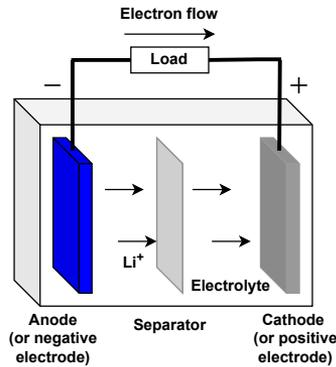
**Figure 2.1:** Schematic illustration of a cell during discharge [9].
