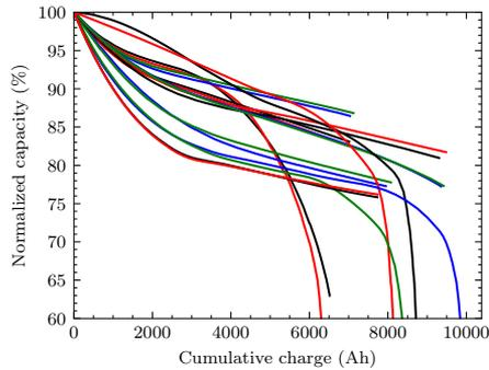
**Figure 3.7:** Normalized capacity fade curves of NMC/graphite-SiO<sub>x</sub> cells in experiment 1, 4 and 5 of Imperial College London dataset [80].
