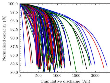
**Figure 3.3:** Normalized capacity fade curves of LFP/graphite cells in the Toyota Research Institute dataset [61] [66].
