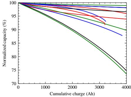
**Figure 3.8:** Normalized capacity fade curves of synthetic NMC/graphite-SiO<sub>x</sub> cells in the Chalmers University of Technology dataset [80].
