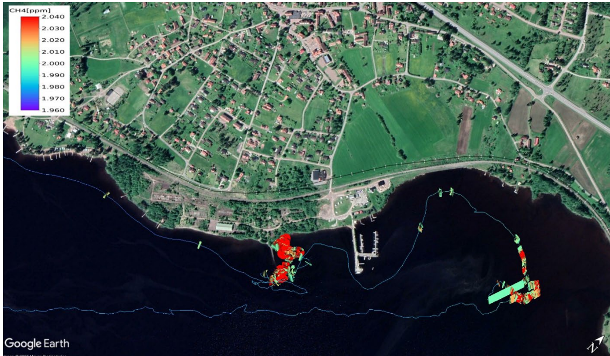
Figure 14. CH_4 concentration mapping at two sources in Vikarbyn: old steamboat pier (left) and Åkersnäsvisken (right).
