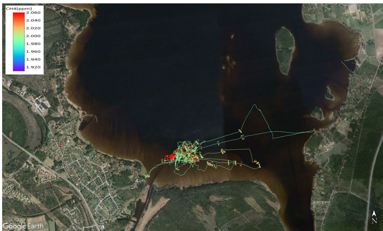
Figure 16. CH 4 concentration mapping in the air above Lake Orsa on June 27, 2024. Two distinct 10×10 m emission hotspots were identified, along with several smaller sources. In these areas, ebullition and diffuse emissions from the water surface were measured, and water samples were collected for isotopic analysis.
