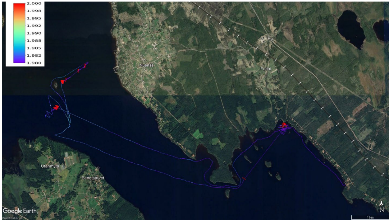
Figure 11. \text{CH}_4 concentration mapping in the air near the northeastern shores of Lake Siljan on June 25, 2024. A distinct \text{CH}_4 source was observed at Fudalsviken, near the harbor inlet, originating from a depth of 5 meters or more. Elevated concentrations were also detected north of Utanmyra on Sollerön.
