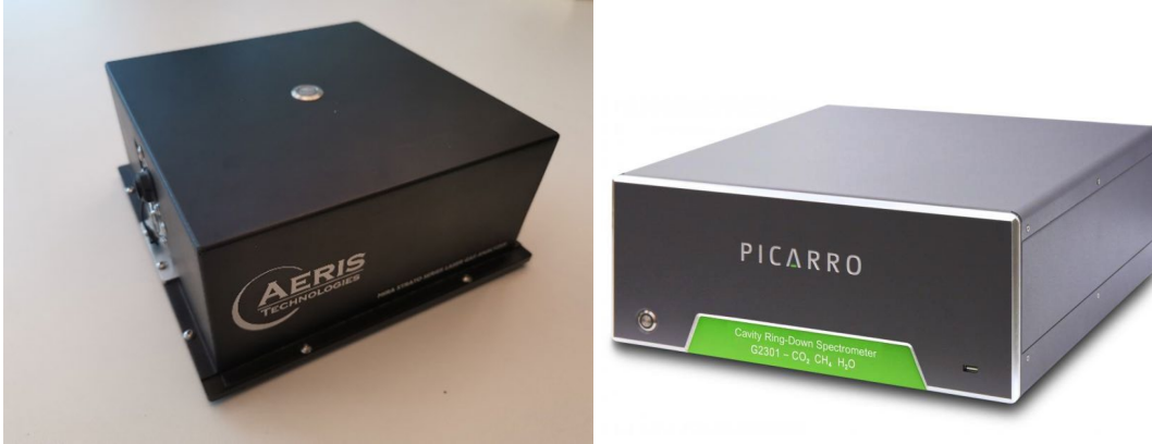
Figure 3. Two Aeris laser sensors (Aeris Strato) were used to measure methane, ethane, and propane, with a sensitivity of 1 ppb and a time resolution of 1 second. An additional sensor, the Picarro G2301, was used to measure carbon dioxide ( \text{CO}_2 ) with a precision of 200 ppb. A third laser sensor, the Picarro G2201-i isotope analyzer, was used in the laboratory. This instrument combines the capabilities of two Picarro \delta^{13}\text{C} carbon isotope instruments for \text{CO}_2 and \text{CH}_4 into a single unit.
