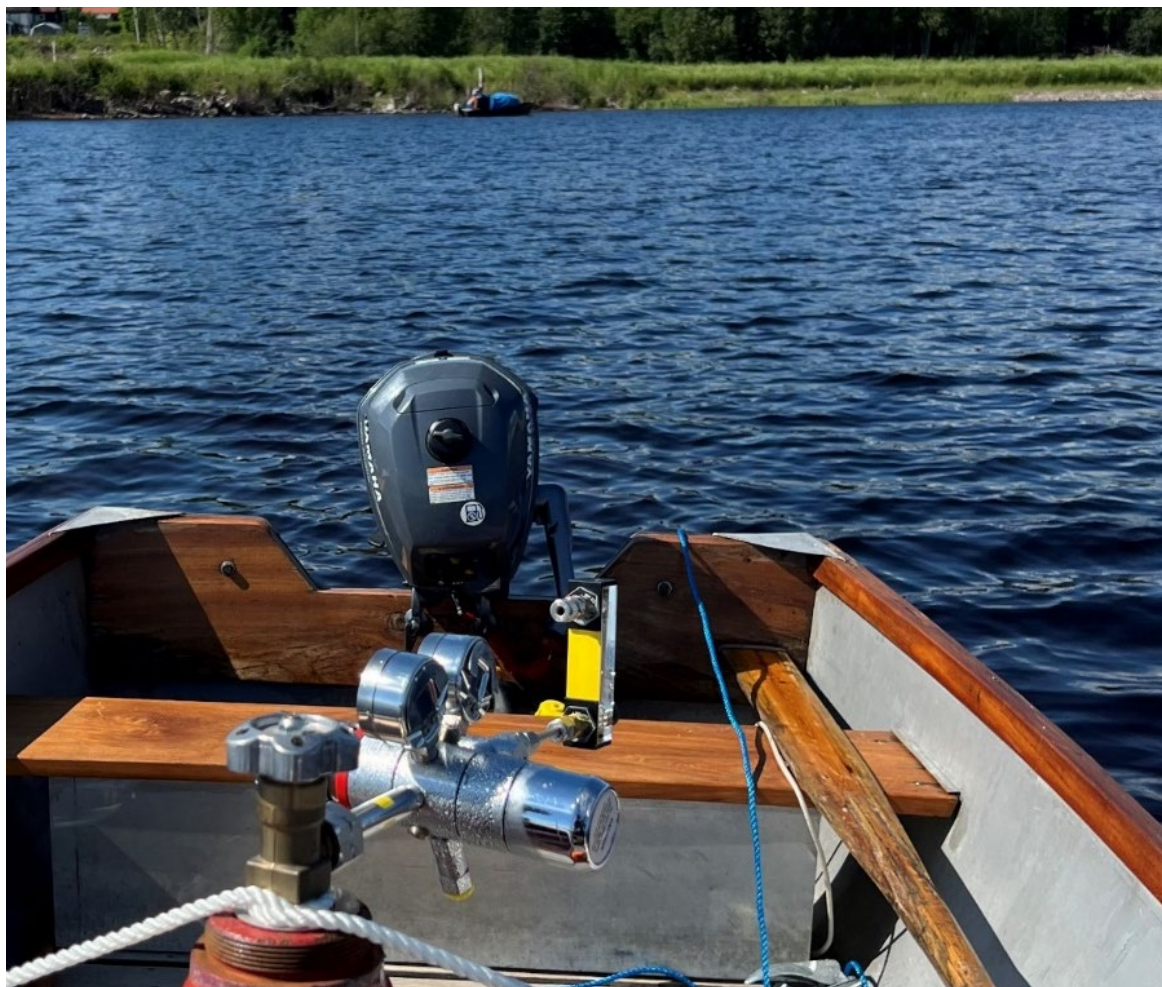
Figure 6. Ethane was utilized as a trace gas and released in a controlled manner near the identified CH 4 leakage sources. This figure shows measurements taken at Vikarbyn, southern Siljan, where the concentrations of CH 4 and ethane were measured approximately 50 meters downstream.
