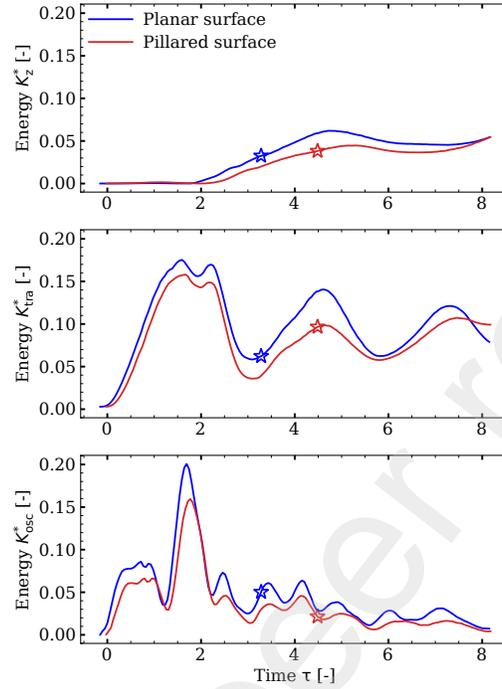
Figure 3: Different components of kinetic energy for a particle-droplet system - comparison between the numerical results obtained for planar and pillared surfaces (S1). The components are the same as those shown in Figure 2. The asterisk symbols indicate the moment of jumping.
