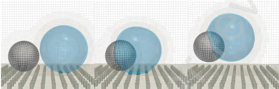
Particle-droplet coalescing and jumping on a pillared superhydrophobic surface.
