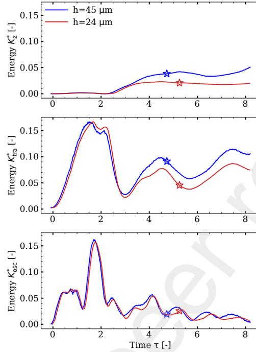
Figure 8: Different components of kinetic energy for a particle-droplet system - comparison between the results obtained for substrates S3 and S5 with different pillar heights (see Table 1). The components are the same as in Figure 2. The energies are normalized by the total released surface energy. The case with higher pillars promotes the superhydrophobic nature of the surface and facilitates the particle-droplet system to jump higher. The asterisk symbols indicate the moment of jumping.
