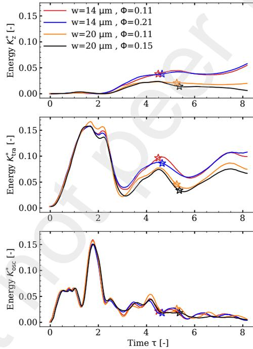
Figure 6: Different components of kinetic energy for a particle-droplet system for S1-S4 (see Table 1). The components are the same as those shown in Figure 2. The energy is dissipated primarily due to the increase of the width of the pillars, with a reduced influence of the pitch sizes. The asterisk symbols indicate the moment of jumping.
