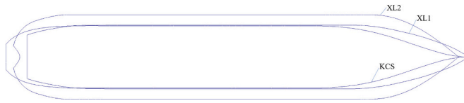
Fig. 16. Comparison of waterline shapes of different ship types.
