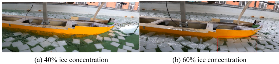
Fig. 6. Ice movement around the ship after activating the air-bubbling system at different ice concentrations.
