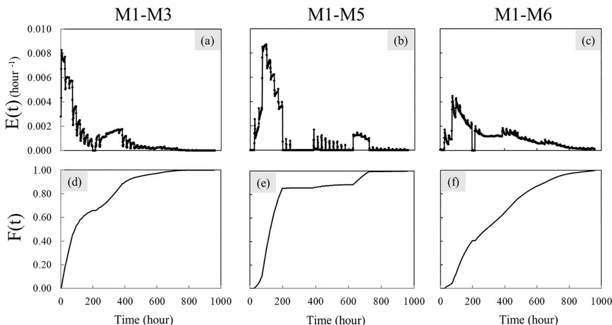
**Figure 3.** Residence time distribution  $E(t)$  and cumulative residence time distribution curve  $F(t)$  of the multi-module systems as measured in filter 1. The operation was interrupted during 264–360 hours due to a technical problem. The zero values in figure b and c indicate lack of data.
