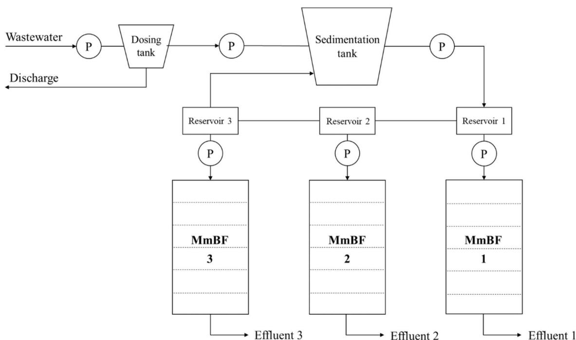
**Figure 2.** Schematic diagram of the experimental setup of the multi-module biochar filters (MmBFs), including the wastewater distribution system. Pump positions are indicated by letter P.
