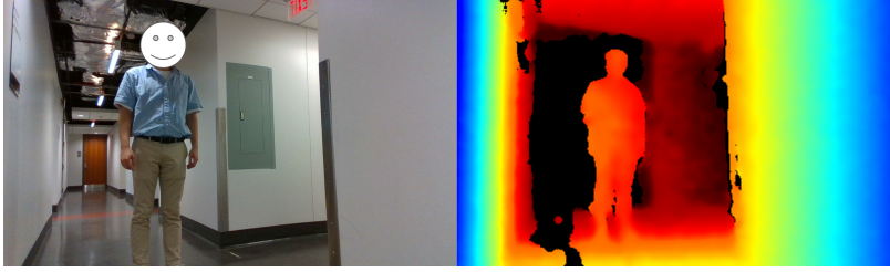
Figure 2.2: Depth image taken by an Intel RealSense depth camera. Each pixel on the depth image (right half) contains a value indicating the distance in the space w.r.t. the camera’s position.
