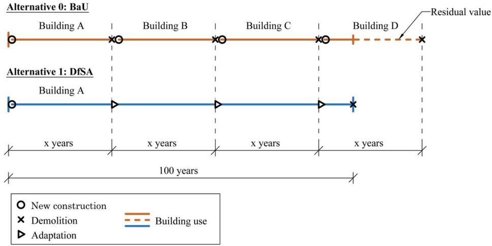
**Figure 2.** Graphical representation of the two alternatives within the time horizon of 100 years.
