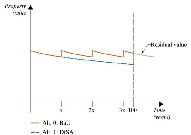
**Figure 3.** Schematic plot of the property value depreciation for the two alternatives, in an example where  $x = 30$  years. As the value depreciates by a percentage each year, the value curves are concave.
