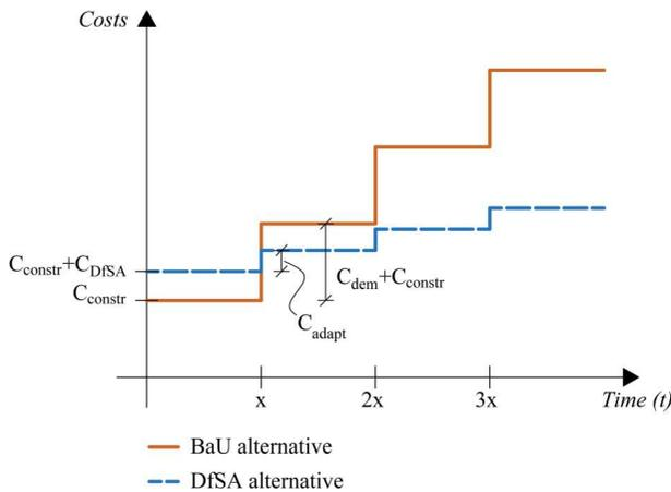
**Figure 1.** Schematic comparison of costs for a DfSA building compared to a BaU alternative, where  $x$  is the average occurrence rate of structural obsolescence.
