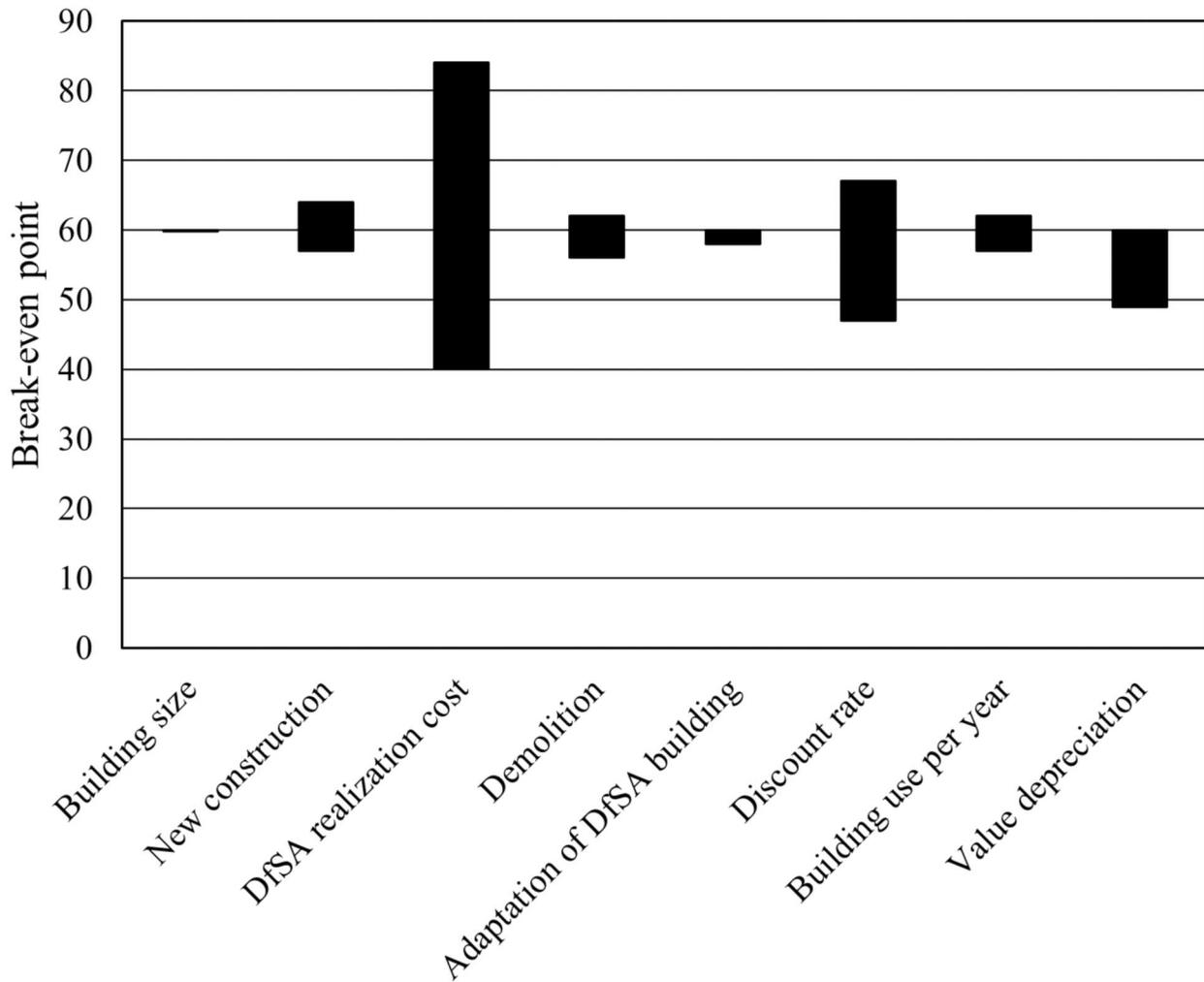
**Figure 7.** Compiled results of the OFAT analysis, showing the break-even point interval for each factor.
