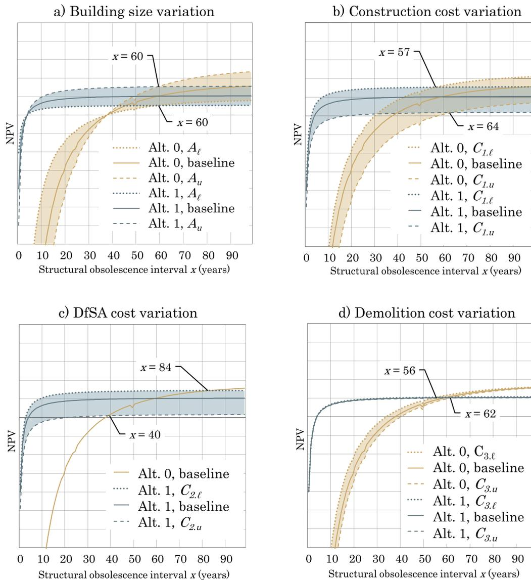
**Figure 5.** Results of the OFAT analysis for (a) building size, (b) construction cost, (c) DfSA realization cost, and (d) demolition cost.
