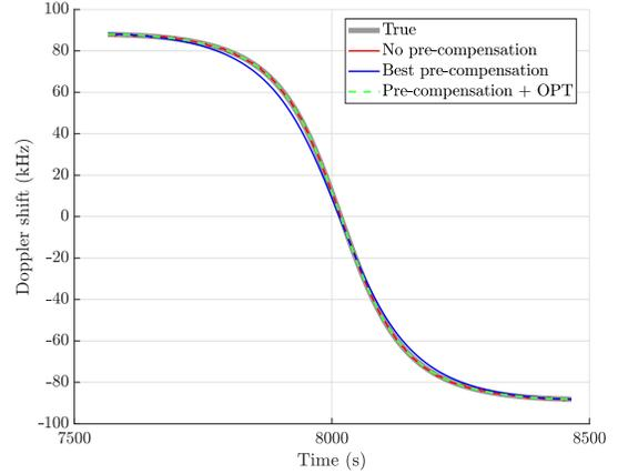
Fig. 2. True and estimated Doppler shifts and best pre-compensation curve for SNR = 15dB and  $f_{s,\text{high}}$ .
