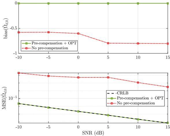
Fig. 5. Bias and MSE of different methods using and  $f_{s,low}$  and varying SNR.
