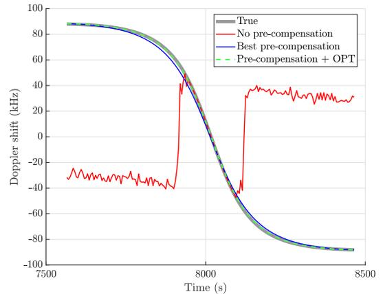
Fig. 3. True and estimated Doppler shifts and best pre-compensation curve for SNR = 15dB and  $f_{s,\text{low}}$ .
