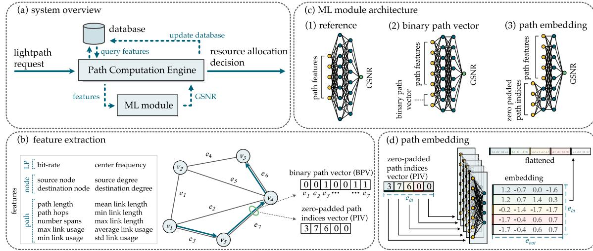
Fig. 1. Summary of the proposed approach, including (a) system overview, (b) feature extraction, (c) ML module architecture, and (d) link-level path embedding.
