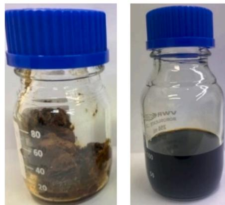
Fig. 9. Left – thermal pyrolysis wax (WAX), Right – catalytic pyrolysis oil (POil).
