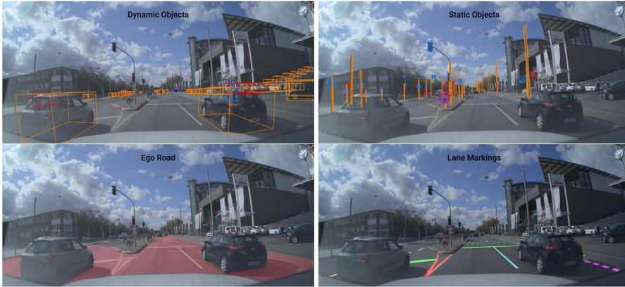
**Figure 2.4:** Examples of different types of annotations, from Zenseact Open Dataset [33].
