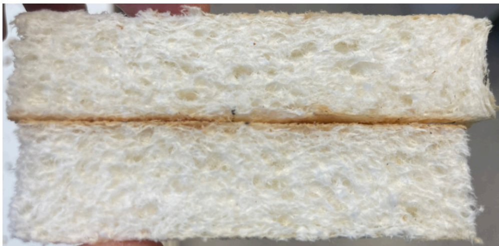
Figure 1.2: Cellulose fiber foam produced from the work in this PhD project.
