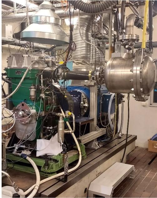
*Figure 2: Heavy duty research engine.*
