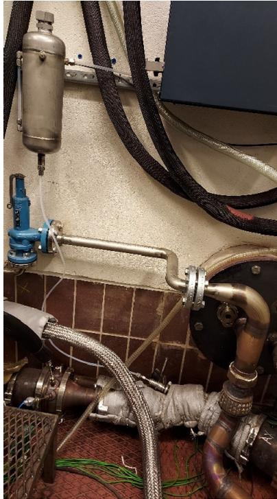
*Figure 7: Urea tank, line to injector and urea injector*
