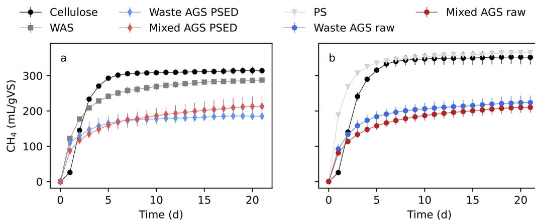
Fig. 1. Biochemical methane potential of the different types of sludge tested in setup I (a) and II (b). Markers and error bars show means and standard deviations. The number of replicates was 2–3 (see supplementary material).
