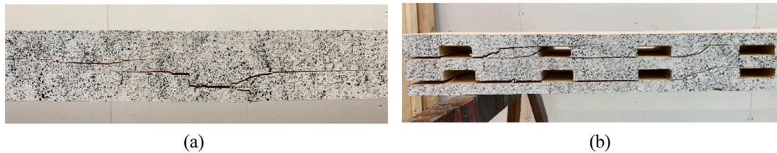
**Fig. 20.** Test results and failure mode of Sample 1 in the four-point bending test: (a) Configuration A, (b) Configuration B.
