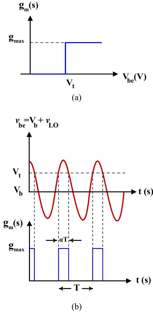
**Figure 2.4:** (a) Transconductance of an ideal transistor. (b) Transconductance waveform [32].
