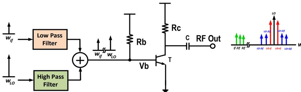
Figure 2.2: Circuit schematic of a single-ended transconductance mixer.
