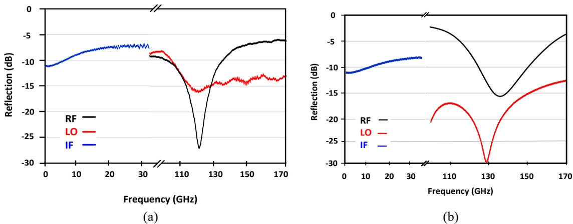
**Figure 4.9:** Measured reflection of IF, LO, and RF ports. (a) Cascode and (b) Darlington pair mixer.
