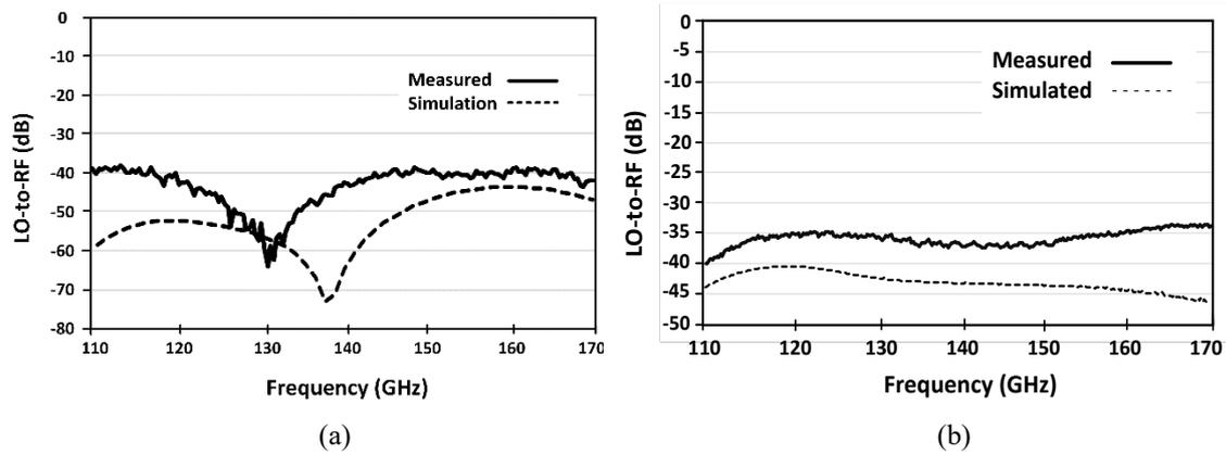
**Figure 4.8:** Measured and simulated LO-to-RF port-to-port isolation. (a) Cascode and (b) Darlington pair mixer.
