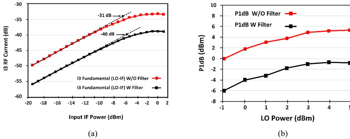
**Figure 3.6:** (a)  $T_3$  Fundamental RF currents ( $I_3$ ) magnitude with and without filter versus input IF power. (b) Mixer's  $P_{1dB}$  with and without filter versus LO power.
