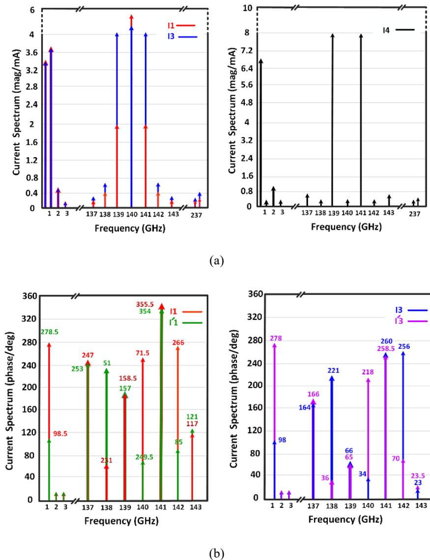
**Figure 3.5:** Simulated spectrum of the mixer current's (a) magnitude (b) phase without the ideal band-pass filter.
