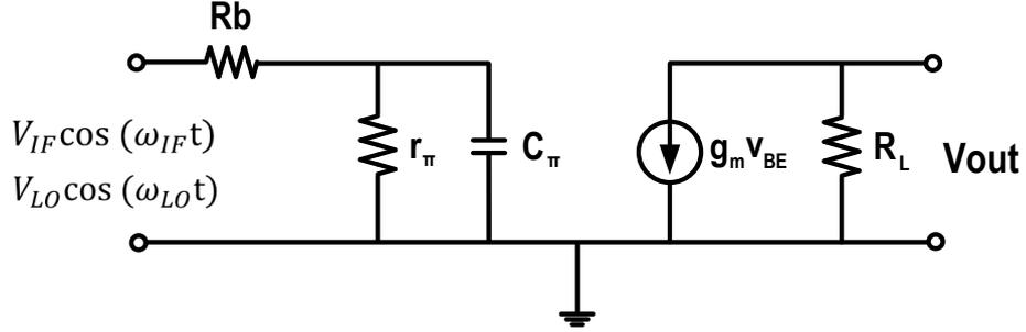
Figure 2.3: Simplified small-signal equivalent circuit of a bipolar transconductance mixer.
