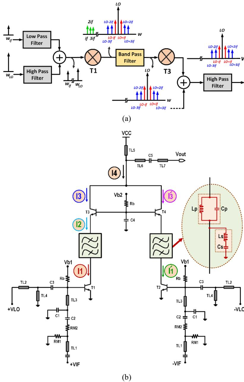
Figure 3.3: (a) Block diagram (system level) (b) circuit diagram of the cascode configuration up-converter with the ideal band-pass filter.
