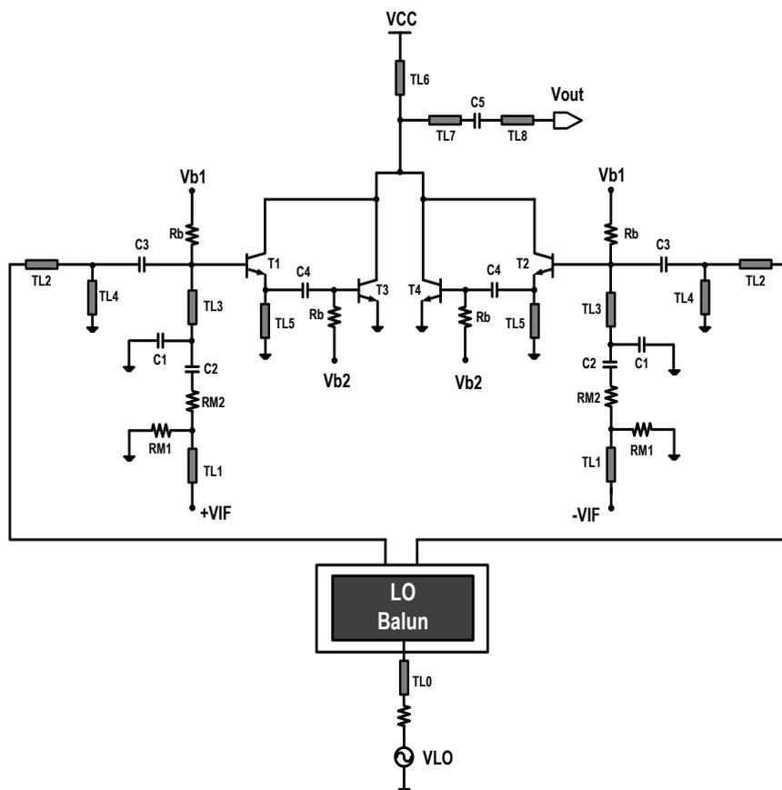
Figure 3.7: Circuit diagram of the proposed Darlington up-converter.
