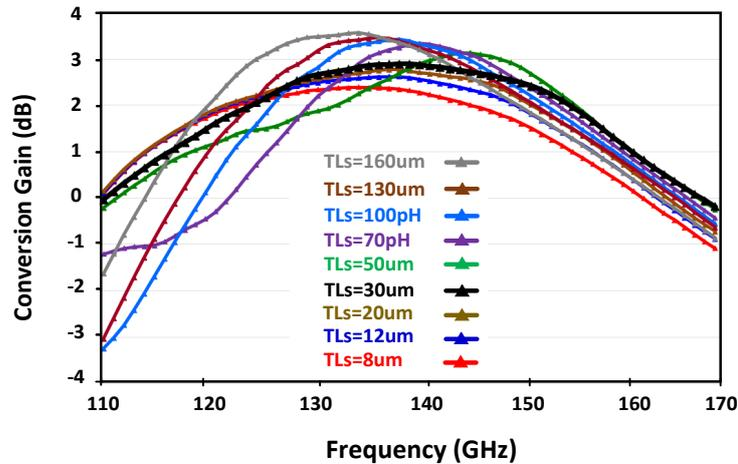
**Figure 3.8:** The conversion gain of the circuit versus LO frequency with different length of the transmission line ( $TL_5$ ).
