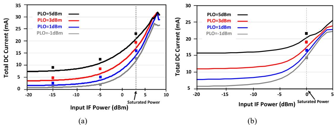
**Figure 4.10:** Simulated (solid) and measured (squares) DC currents of the mixer versus input IF power at 138 GHz LO and 2 GHz IF frequency for (a) cascode mixer and (b) Darlington pair mixer.
