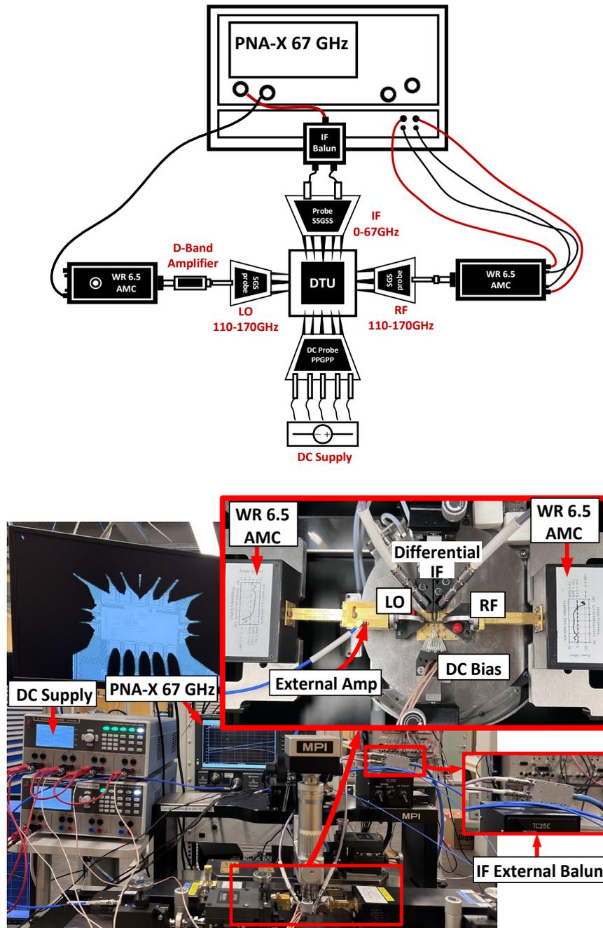
Figure 4.2: Measurement setup for CG and output power.
