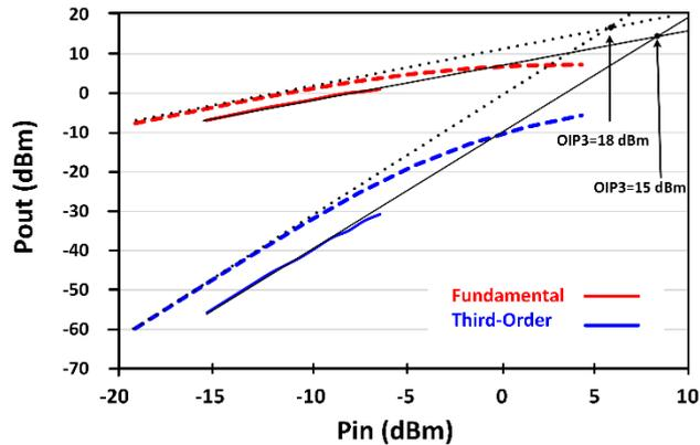
**Figure 4.7:** Measured fundamental and  $IM_3$  tone output power versus input power of the proposed mixer at LO frequency of 140 GHz and IF frequency of 2 GHz with 100 MHz tones space. Simulation results (dashed line) are also included.
