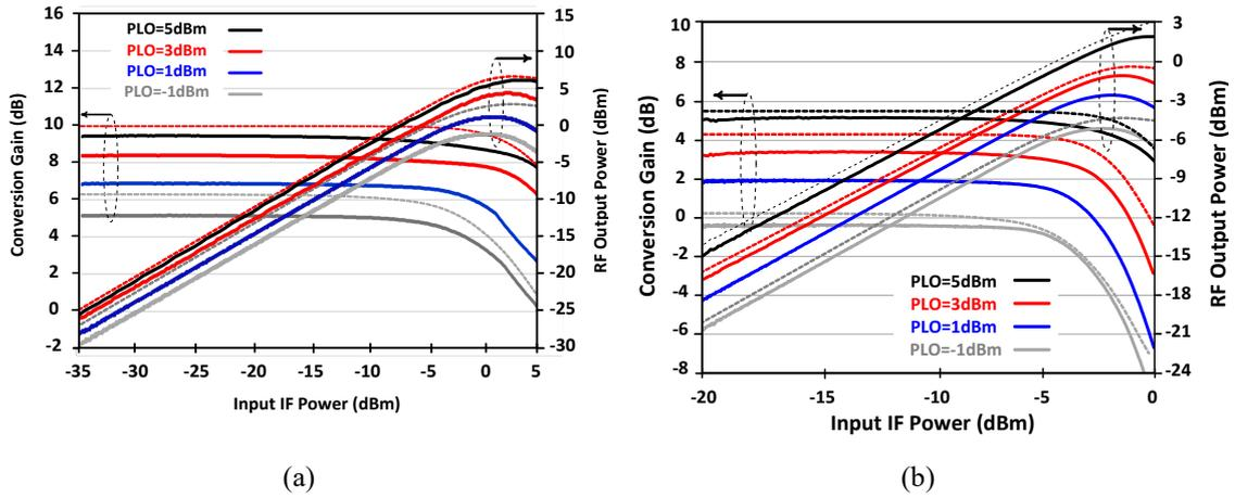
**Figure 4.3:** Measured conversion gain ( $CG$ ) and output RF power versus input IF power with -1, 1, 3 and 5 dBm LO at 140 GHz. Simulated (dashed line)  $CG$  and output power are also included. (a) Cascode mixer - and (b) Darlington pair.
