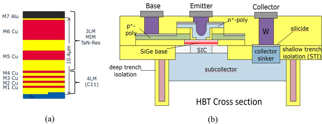
**Figure 2.1:** (a) 7-layer metallization (b) Cross section for an NPN transistor [30].
