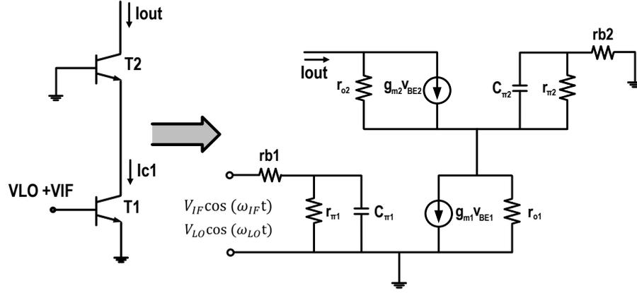
**Figure 3.2:** Simplified small-signal equivalent circuit of a bipolar transconductance mixer with the cascode structure.
