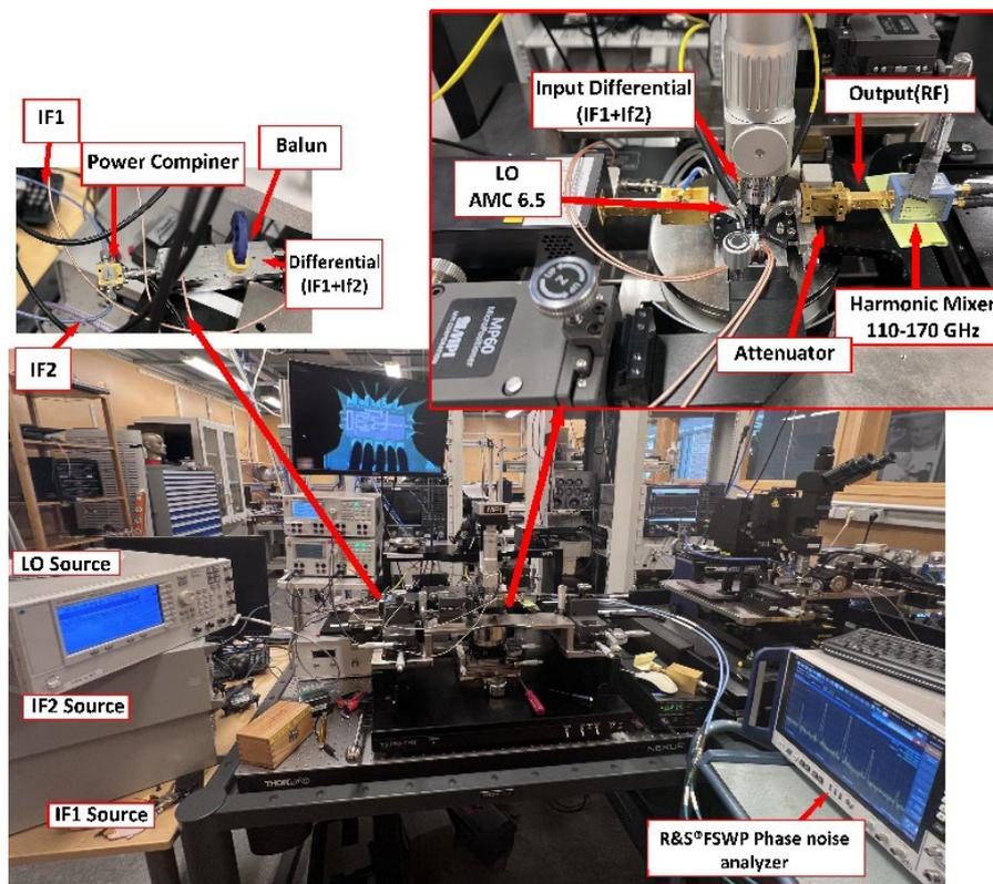
Figure 4.6:  $OIP_3$  Measurement setup.
