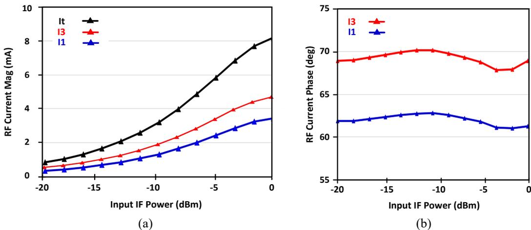
**Figure 3.10:** Simulated RF currents  $I_1$ ,  $I_3$  and  $I_t$  versus  $P_{if}$ . (a) magnitude (b) phase at LO frequency 140 GHz, IF frequency 2 GHz, LO power 5 dBm.
