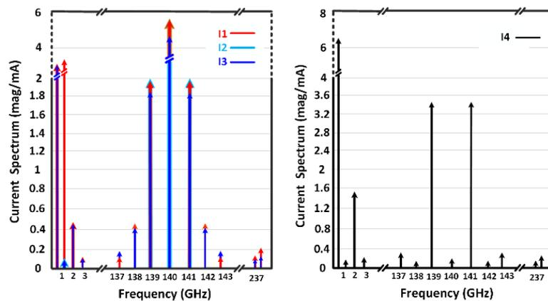
Figure 3.4: Simulated spectrum of the mixer currents magnitude with the ideal band-pass filter.
