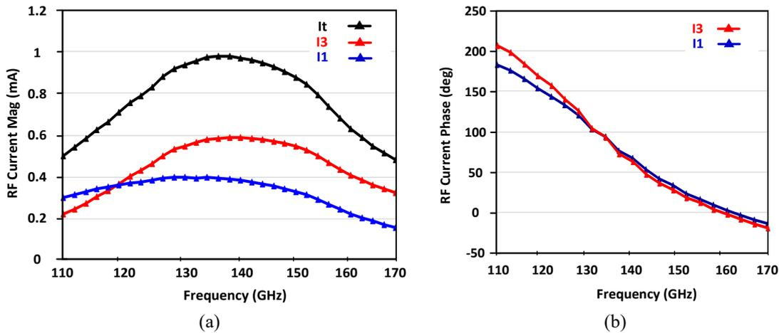
**Figure 3.9:** Simulated RF currents  $I_1$ ,  $I_3$  and  $I_t$  versus  $f_{LO}$  (a) magnitude (b) phase at IF frequency 2 GHz, LO power 5 dBm.
