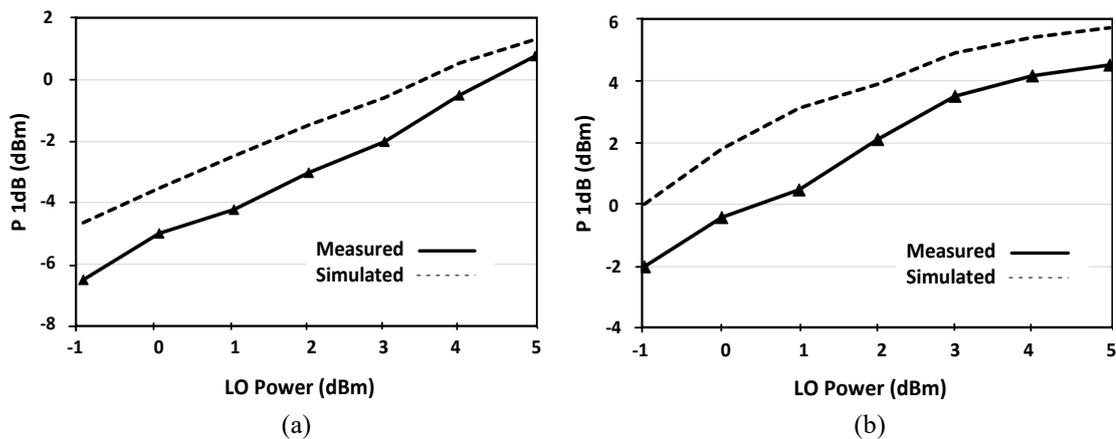
**Figure 4.5:** Measured and simulated  $OP_{1dB}$  versus LO power at LO frequency of 138 GHz and IF frequency of 2 GHz for (a) Cascode mixer - and (b) Darlington pair.
