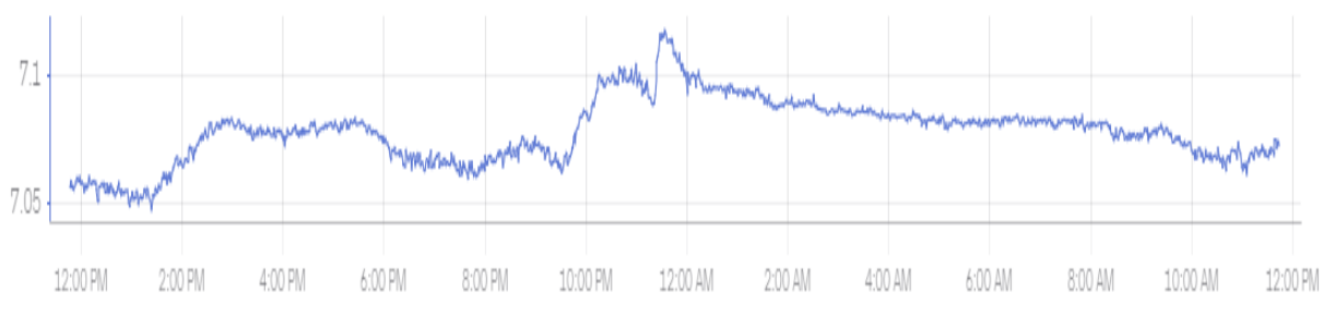
Figure 5. Biodigester pH data remotely captured by pH sensors and sent to remote monitoring offices.
