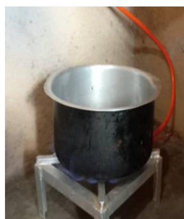
(c) biogas burner (stove) at kitchen end
