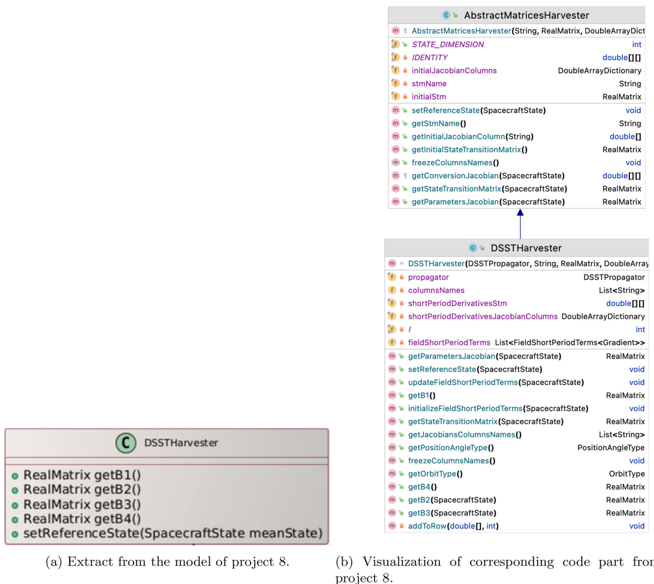
Fig. 3 The superclass AbstractMatricesHarvester with its attributes and operations from the code are hidden in the model
