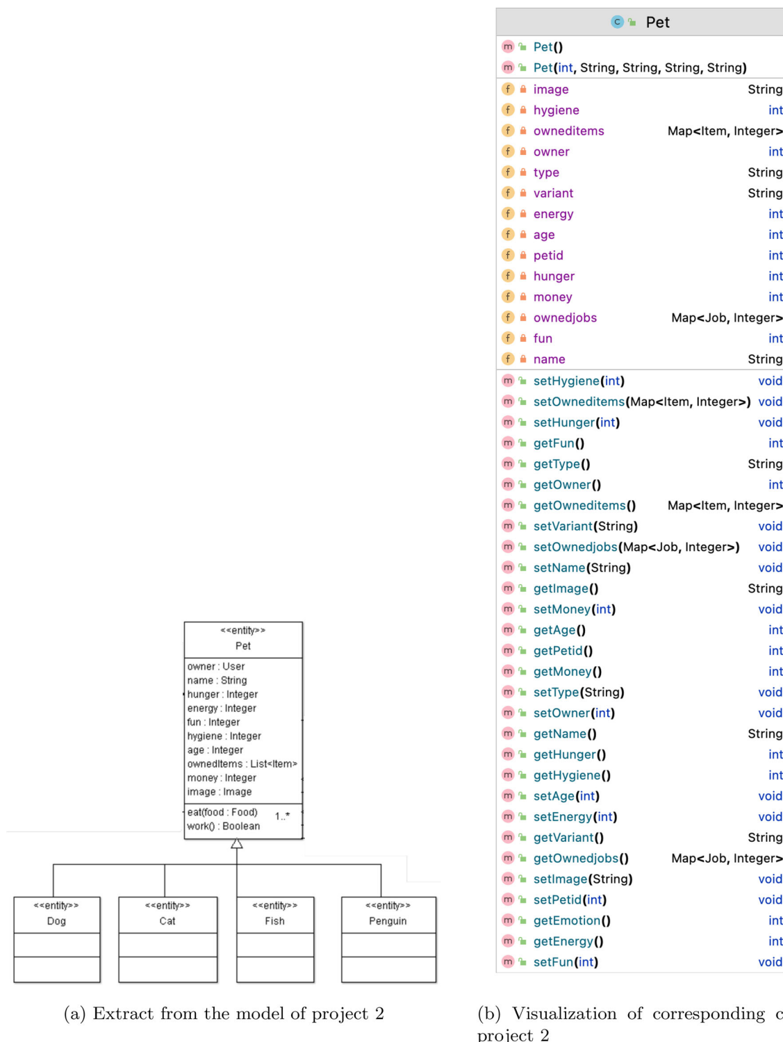
Fig. 9 Subclass pretense: The subclasses of Dog, Cat, Fish, and Penguin of the inheritance structure with the superclass Pet and an operation eat(food: Food) in the model, which are both not present in the source code
