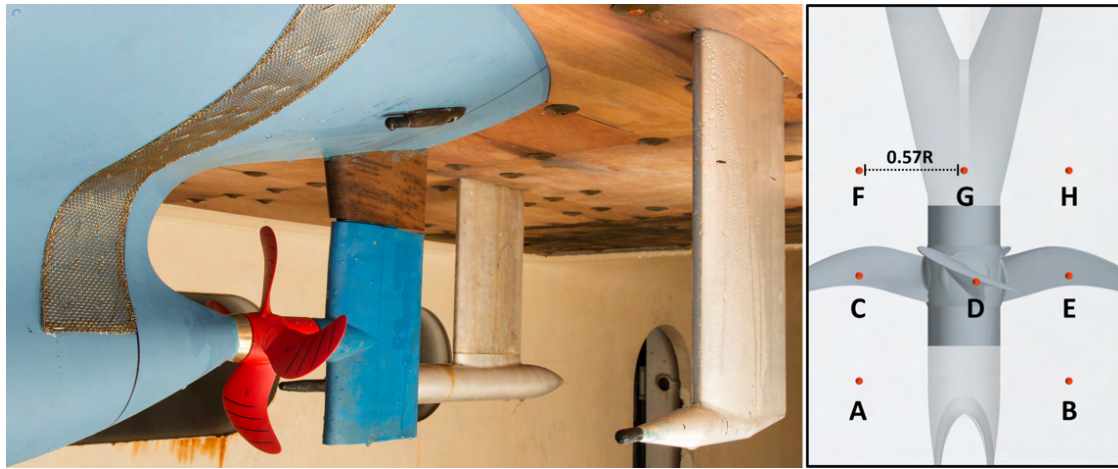
Figure 3.9: Ship mounting in RISE cavitation tunnel (left) and top view for the pressure transducers placement during the model tests.
