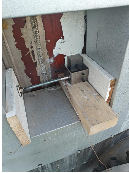
Figure 5.4: The transducer mounted to the impregnation vessel.
