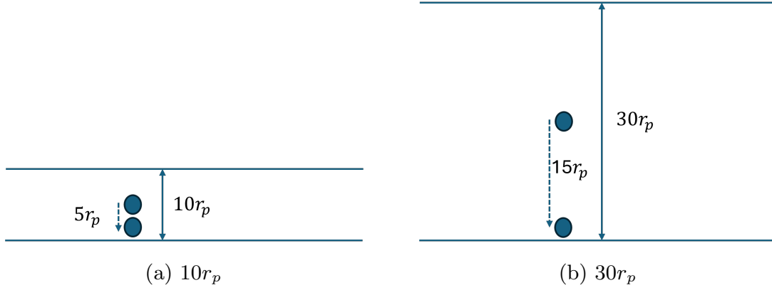
Figure 4.3: The two domains used in the multiscale simulations of Brownian particle migration: (a) domain with walls separated by a distance of 10r_p in the z direction, (b) domain with walls separated by 30r_p .
