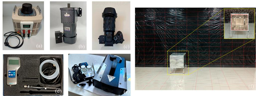
**Figure 2.** Experimental instruments and devices: (a) voltage regulator (TDGC20K, CNCQIANG, Wenzhou, Zhejiang, China), (b) speed-regulating motor (TGU-40K, TVT, Wenzhou, Zhejiang, China), (c) high-speed camera (ILCE-7CL, Sony, Tokyo, Japan), (d) air velocity probe (Model 65Ser, KANOMAX, Shenyang, Liaoning, China), (e) smoke generator (FM1500, Jieyoong, China), and (f) heat source device (Handmade, in which the red dotted line indicates the edge).
