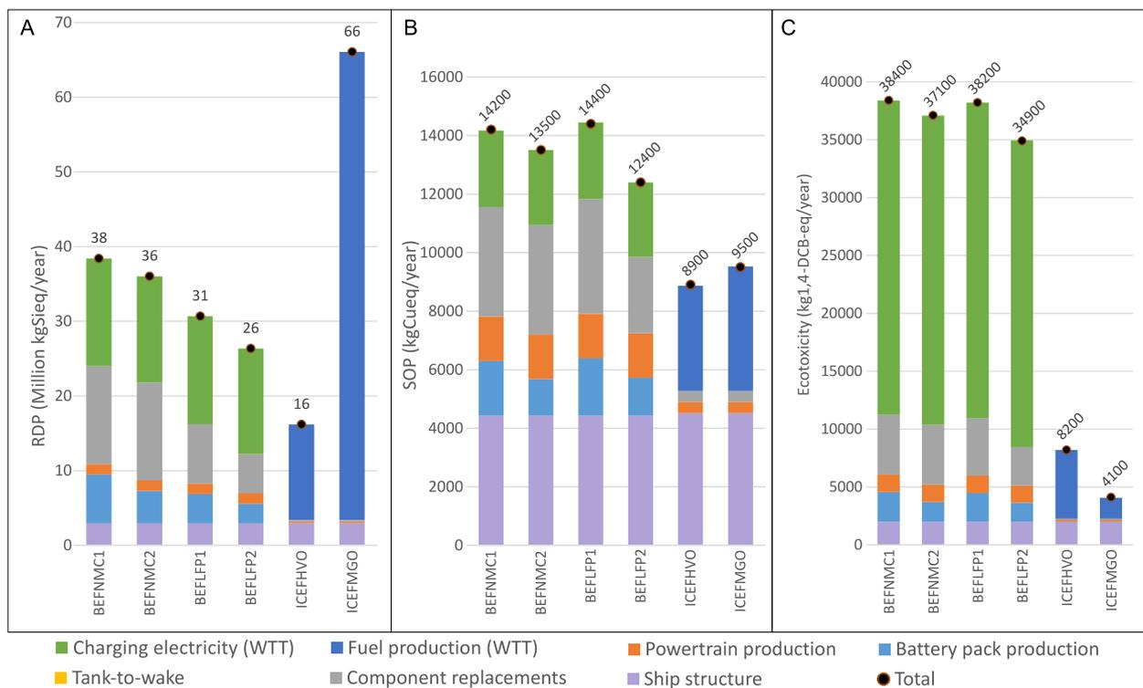
Fig. 7. Impact assessment results for two indicators covering mineral resource depletion – the crustal scarcity indicator in RDP providing a potential for long-term scarcity and the surplus ore indicator (SOP) providing a short perspective on resource availability – and freshwater ecotoxicity. Common for all these impact categories is that the BEF options generally have a higher impact than ICEFHVO or ICEFMGO options, except for the CSP of the ICEFMGO.
