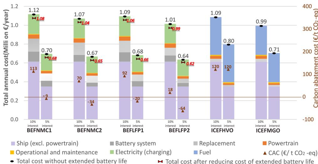
Fig. 8. LCC results for the six cases assessed for the functional unit annual operation of the ferry.
