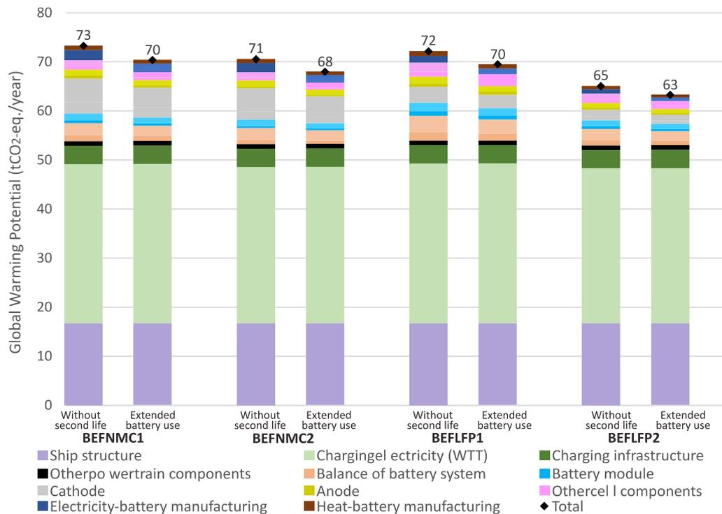
Fig. 4. Breakdown of the GWP for the BEF options including the scenario where a share of the burden from battery production is allocated to a second life application (right side bar for each option) resulting in lower impact from the ferries. Lighter color in each battery component represents impact associated with replacement.
