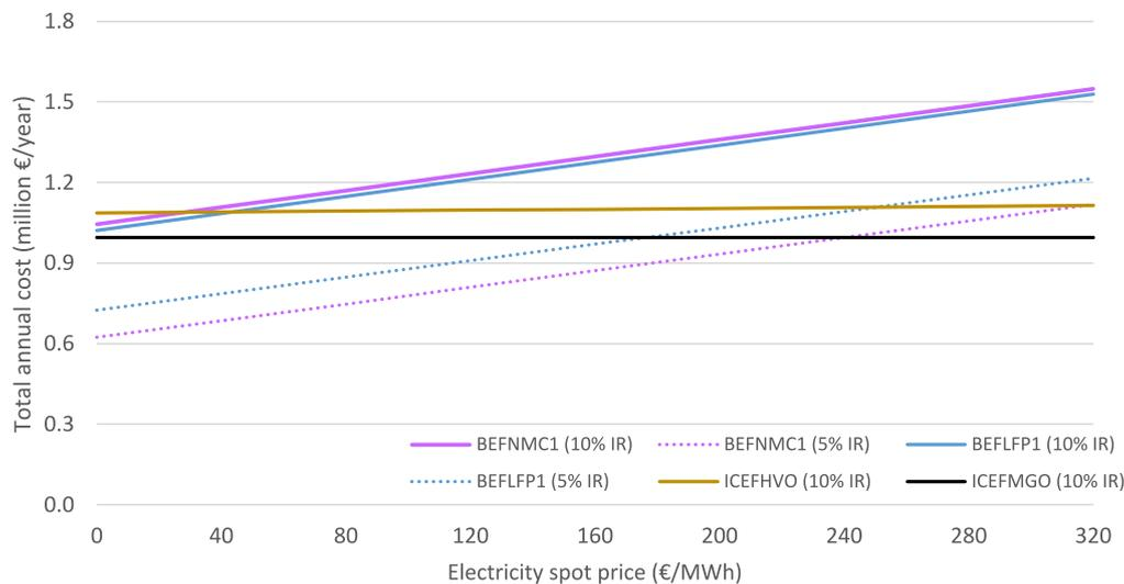
Fig. 9. Sensitivity analysis on total cost as function of average spot electricity price on total annual cost including all life cycle stages. IR-Interest rate.
