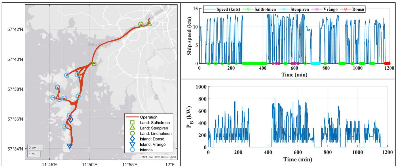
**Fig. 1.** Operation of case study vessel. A.) Route during 4 days in autumn, B.) speed in the selected route, C.) Brake power.
