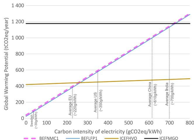
Fig. 5. Sensitivity analysis of the cradle to grave global warming potential (GWP) for the ferry as a function of the carbon intensity of electricity used (0–800gCO<sub>2</sub>eq/kWh). It may be noted that the various electricity mixes indicated in the figure are the present carbon intensity of the regions reported in IEA [65] and not prospective mixes.
