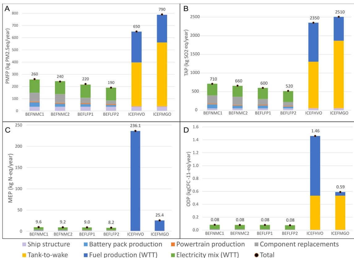
Fig. 6. LCA results for the impact categories that have a lower impact for BEFs than HVOICE and MGOICE. PMFP: Particulate matter formation potential, TAP: Terrestrial acidification potential, MEP: Marine eutrophication potential, ODP: Ozone depletion potential.
