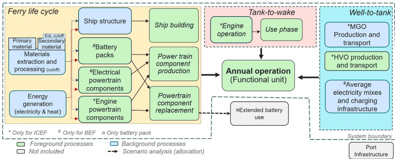
Fig. 2. Life cycle system boundary used in the study: ferry life cycle, tank-to-wake, and well-to-tank. The foreground data combines calculated data with data from previously published works, while the background data is from Ecoinvent v3.9.
