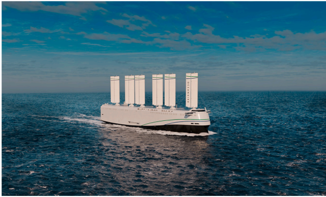
Fig. 1. Concept design of the Oceanbird wingsail ship (Oceanbird, 2021).
