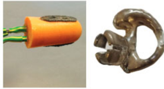
Figure 7. In-ear EEG using wet and dry electrodes, respectively. Adapted from [24,25].
