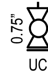
Fig. 14. An example of a Ball valve with a size indicated next to it.
