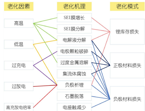
图6 (网络版彩图)锂离子电池老化模式、机理与影响因素 Figure 6 (Color online) The aging modes, mechanisms, and influencing factors of lithium-ion batteries.
