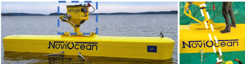
Figure 3.6: NoviOcean WEC prototype model (scale 1:2) (Novige, 2023). The water turbine is in the blue box and the hydraulic cylinder in the dashed white box.
