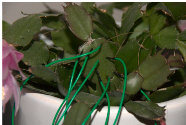
Fig. 1. Electrodes in Schlumbergera cactus used for reservoir computing (Adamatzky et al., 2017b).
