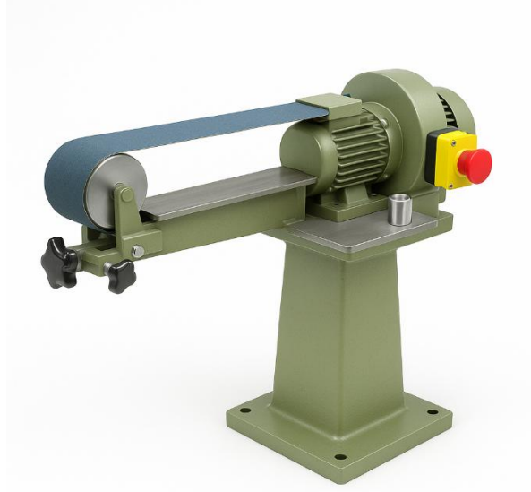
Figure 7) grinding band used to polish the metal strips.
