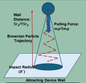
Simulation of Brownian particle pulled towards a wall using a constant force
