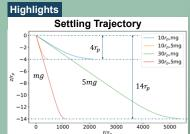
Hydrodynamic hindrance increases close to the wall slowing the particles down
