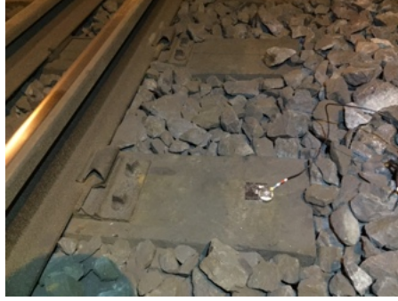
Figure 3.1: Accelerometer position on the sleeper.
