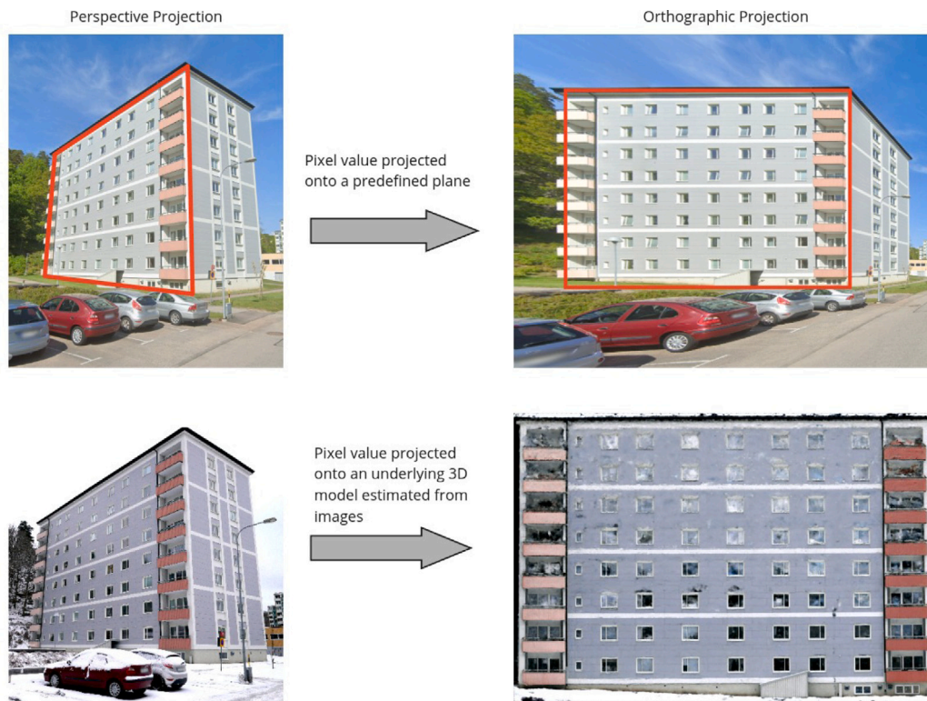
Fig. 1. Comparison of perspective images with proposed orthographic images for both sparse images (first row; from Google Street View) and dense images (second row; using a perspective camera).
