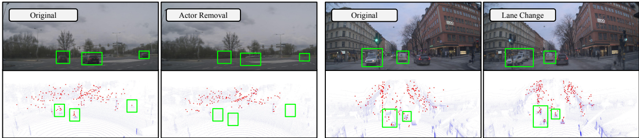
Figure 1. NeuRadar generates radar point clouds alongside camera and lidar data for novel viewpoints and altered scenes. This figure illustrates images, radar point clouds (in red), and lidar point clouds (in blue) generated by NeuRadar for two sequences in ZOD.
