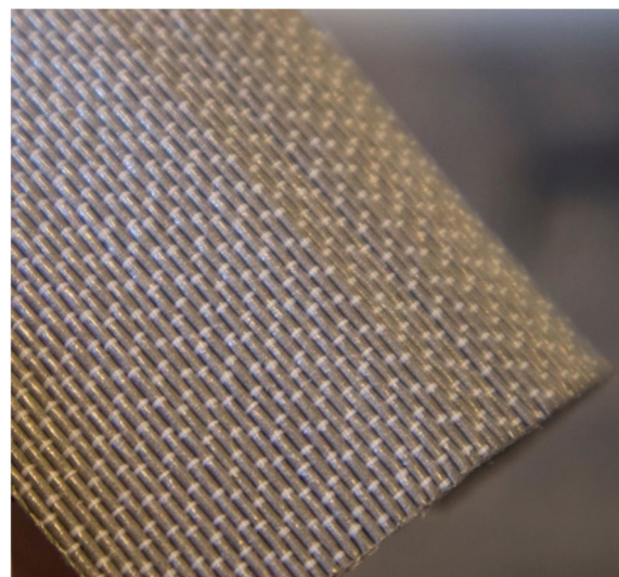
Fig. 1 The Texray textile material, 0.25 mm Pb equivalence
