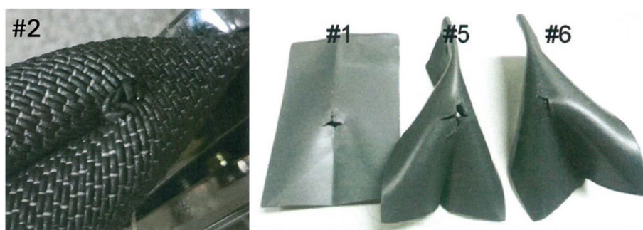
Fig. 2 Images of Bally Flexing tester. Sample #2 is the Texray 0.25 mm Pb eq. after 300,000 cycles. The samples #1, #5 and #6 are attenuating rubber-like sheet materials after 25,000 cycles
