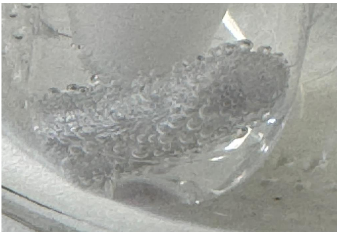
Figure 3: Rapid hydrogen evolution on the surface of the R2 alloy in CW.
